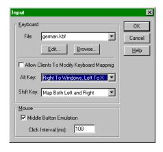
In the list field "Alt key", select "**Right To Windows**, **Left To X**". Close with "OK". Restart user interface of the control unit.
